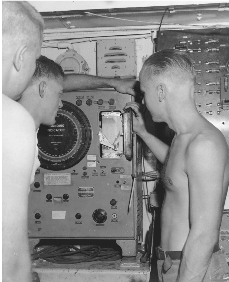
Figure 3. The echo sounder, seen here being examined by scientists below deck, was the basic instrument for mapping the depth of the sea floor. (Courtesy of the Woods Hole Oceanographic Institution.)
